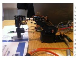
To demonstrate how the ebbits platform can handle and respond to data from devices, a temperature sensor was attached to the robot. When the temperature was raised above 30°C, simulating the temperature in the robot's cooling system, the robot stopped immediately and issued a warning signal to the operator central, located in Sweden.
