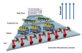
Management of real-time data will be demonstrated in the automotive manufacturing setting, where real-time data from units, components and sensors are pulled from the underlying layers of the factory into the plant level to be used in online ebbits services for online production management, energy monitoring and maintenance performance.
